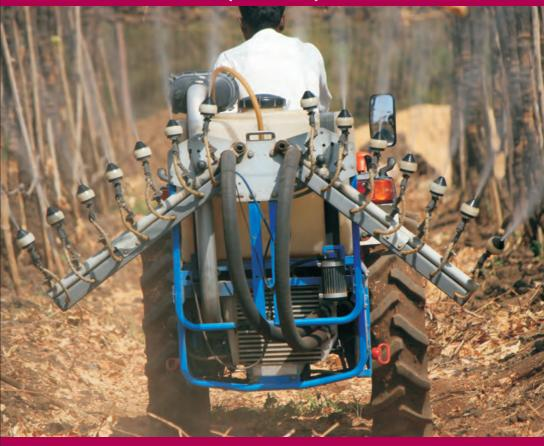
Electrostatic Spraying Systems ,Inc,USA(ESS) manufactures wide range of Electrostatic Sprayers for Horticulture and Row Crops. The heart of the air assisted electrostatic sprayer is the patented "Air Atomising Induction Charging-MaxCharge Nozzle",which was invented by Dr.Edward Law of the University Of Georgia. ESS sprayers are being used in most Grape growing countries of the world for Table as well as Wine Grapes to spray Pesticides and PGRs.
