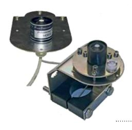
The IM506D Pyranometer is designed for field measurements of global solar radiation in agricultural, meteorological and solar energy studies. In clear, unobstructed daylight, the Pessl Instruments pyranometer has favourable results compared to the first class thermopile-type pyranometers, but is priced at just a fraction of the cost.
