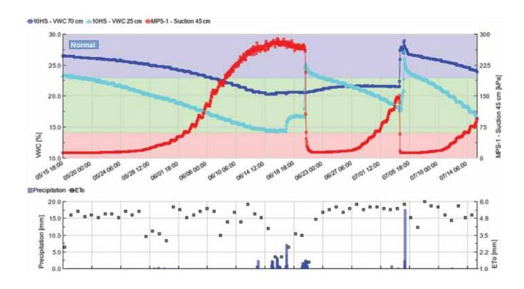
Example of soil moisture monitoring in vineyard (Pinot Noir - South Tyrol - Italy). The first graph reports data of volumetric water content (VWC) at two different depths and of suction. The graph on the bottom shows data of precipitation and ETO.
