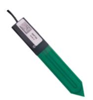
The 100SMT is an accurate soil moisture probe for monitoring volumetric water content and soil temperature. The oscillation frequency is related to the dielectric permittivity of the surrounding medium. The relation between the permittivity and the soil moisture depends on the soil type and the soil temperature, therefore all dielectric measurement techniques require a material and temperature dependent calibration for highest precision.
