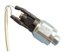
Simple and robust construction and adjustable switching point through headless screw make pressure switch suitable for use with compressed air, hydraulic oil, oil emulsions and water. It is adjustable form 1 to 10 bar or 0.2 to 2 bar. The main purpose of this sensor is to control/check the correct performance of the irrigation system.
