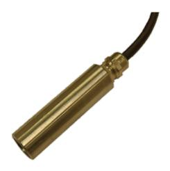
The LMP305 is an accurate but cost effective stainless steel submersible water level sensor that can be connected to iMETOS stations with the precision of +/-3 % within the measurement ranges. Sensor has an integrated Barometric sensor module to increase the precision. Pressure (Measuring) ranges: 0 mWC up to 5 mWC (other distances on request). Water level special cable is also available.
