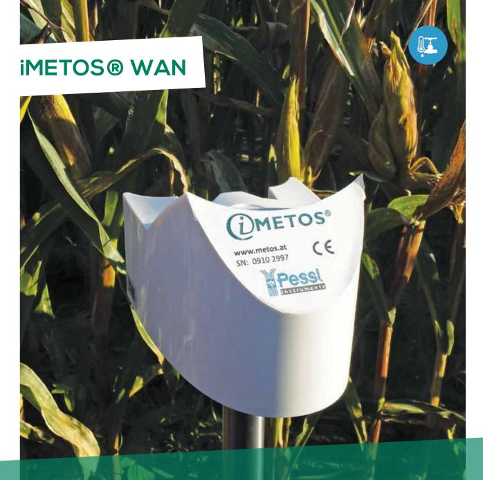
The iMETOS® WAN (WIRELESS ACTIVATOR NODE) comes in an IP67 case, with a LI-Battery and can operate for about 7 years. Using the wireless interface, iMETOS WAN can switch most standard time-based irrigation controllers and any other commands which changes the status.
