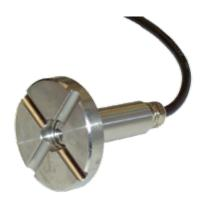
ET-250 is a highly accurate stainless steel submersible water level sensor used for Class A Evaporation pans to be connected to iMETOS stations. Highest precision is reached with Keller sensor technology, water temperature compensation and integrated barometric sensor module. Due to its innovative design, most mechanical Class A pans can be retrofitted with automatic ET measurements. It measures with 0.2% accuracy.
