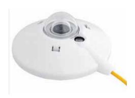
The CMP 6 pyranometer is intended for routine global solar radiation measurement research on a plane/level surface. Fully compliant with ISO 9060:1990 specification for a First Class pyranometer, the CMP 6 features a sixty-four-thermocouple junction (series connected) sensing element. The sensing element is coated with highly stable carbon based non-organic coating, which delivers excellent spectral absorption and long-term stability. It is reliable in all weather conditions.
