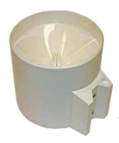
The mechanic consists of a small magnet, which moves past a metallic switch and opens or closes the circuit. The double spoon tips left or right and does not lose any water due to a very fast switching mechanics. The resolution with a surface of 200 cm2 is 0.2 mm, while the resolution with the 80 cm2 is 0.5 mm. Heating for rain gauge can also be included.
