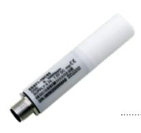
CO2 sensors, with patented auto-calibration for climate technology and building management are based on a 2-source, 2-beam process. This technology offers long-term stability, ensured by the tested and trusted NDIR CO2 measurement cell. The miniature design of CO2 sensor is ideally suited for applications in the environmental fields indoor as well as outdoor.
