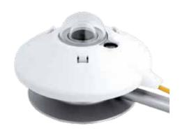
The CMA albedometers are double pyranometers that measure both global and reflected solar irradiance in one instrument. CMA albedometers are suitable for measuring global radiation and/or albedo over many different types of surface. The upper pyranometer measures incoming global solar radiation and the lower sensor measures solar radiation reflected from the surface below. CMA 6 is constructed from two CMP 6 pyranometer sensors.
