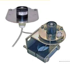
Photometry or Luxmeter IM508D refers to the measurement of visible radiation (light) with a sensor having a spectral responsivity curve equal to the average human eye. The sensor is used to measure lighting conditions where the eye is the primary receiver, such as illumination of work areas, greenhouses, interior lighting etc.
