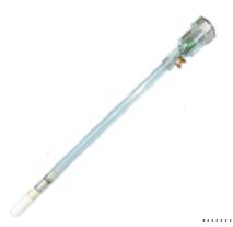
The instrument measures soil water tension in centibars (cbar) or kilopascals (kPa). This value represents the energy a plant's root system uses to draw water from the soil. Understanding soil moisture activity helps the user make informed irrigation scheduling decisions, resulting in improved yield and quality while reducing water, fertilizer, labor and energy costs.
