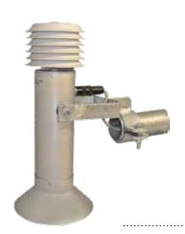
Ultrasonic snow depth sensor is used for non-contact measurement of snow-depth in extreme conditions with ultrasonic sensors. The sensor is characterized by its high level of operating reliability, low energy consumption and ease of use in the field.
