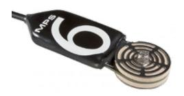
The MPS-6 is a matrix water potential sensor that provides long term, maintenance-free soil water potential and temperature readings at any depth without sensitivity to salts. The range of the MPS-6 goes from field capacity to air dry (-9 to -100,000 kPa). Lab and field tests indicate that it can make accurate measurements of water potentials at least as dry as permanent wilting point.
