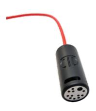
The Decagon CTD-10 sensor is a low cost, accurate tool for monitoring of water level, electrical conductivity, and temperature in both ground water and surface water. The sensor utilizes a vented pressure transducer to obtain accurate water level measurements from 0 to 10 m while removing the effects of barometric pressure. With a range of 0 to 120 dS/m, the CTD sensor has the ability to make accurate electrical conductivity measurements in a broad range of applications.
