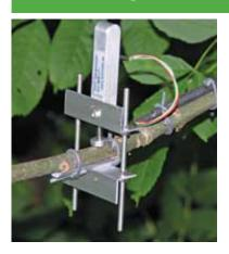
Dendrometers are sensors for continuous measurement of plant growth (changes of the plant diameter). The dendrometer allows us to record the plant parameters using the same time interval, as environmental parameters. The data, therefore, allows the direct assignment of plant responses and stress to environmental influences. Dendrometers are a cost-effective and useful tool for ecophysiological studies.
