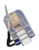
The leaf wetness sensor works by measuring the conductivity in a filter paper. The filter paper is held between two stainless steel electrodes in a transparent holder. The use of transparent Lucite plastic as a holder reduces the warming up of the sensor when it is exposed to direct sunlight.
