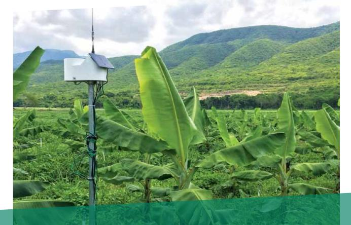
The wireless iMETOS® ECO D3 is a solar panel and battery powered data logger with rain gauge and sensors for water level, temperature, soil moisture, salinity, etc., designed to work in harsh conditions and in all climate zones. The system has a fully integrated UMTS/CDMA modem for direct communication with the FieldClimate.com platform and can handle up to 400 sensors through the intelligent sensor bus system.
