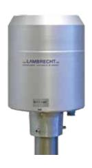
The mechanic consists of a small magnet, which moves past a metallic switch and opens or closes the circuit. The double spoon tips left or right and does not lose any water due to a very fast switching mechanics. The resolution with a surface of 200 cm2 is 0.2 mm, while the resolution with the 80 cm2 is 0.5 mm. Heating for rain gauge can also be included.
