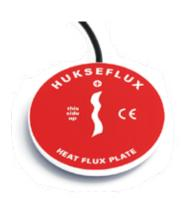
LP02 serves to measure the heat that flows through the object on which it is incorporated or in which it is mounted. The actual sensor in LP02 is a thermopile. It measures the differential temperature across the ceramics-plastic composite body of LP02. Working completely passively, LP02 generates a small output voltage proportional to the local heat flux.
