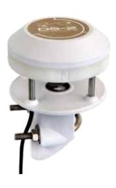
The DS-2 is a research-grade two-dimensional sonic wind sensor, built specifically for agricultural, forestry, and environmental research applications. A lower wind speed threshold makes it especially well suited for measuring wind within plant canopies, where wind speeds are often below the threshold of a cup wind sensor.
