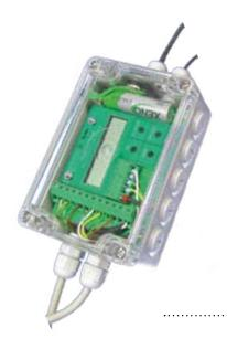
The EC500PH EC & PH Interfacebox is a measuring device with display in IP65 Box to be integrated into any iMETOS sensor chain interface for continuous EC & PH measurements in water. The outstanding design allows the use of the majority industry standard EC & PH sensors. On the display, the actual reading can be seen. With the built in calibration mode, all sensor readings can be calibrated and checked from time to time.
