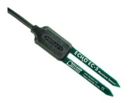
The EC-5 is a basic, reliable and low cost soil moisture sensor. The EC-5 determines volumetric water content (VWC) by measuring the dielectric constant of the media using capacitance/frequency domain technology. Its 70 MHz frequency minimizes salinity and textural effects, making this sensor accurate in almost any soil or soilless media. It is just 5 cm long, and has a 0.3 L measurement volume.
