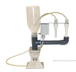
The highly reliable and experienced SMT 172 (or Pt1000) is built in a waterproof housing, covered by cotton tissue and wetted by water. This is the most accurate way to directly determine the dew point.
