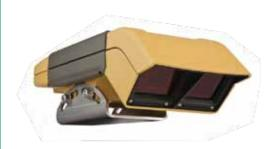
Topcon's CropSpec is a real-time integrated crop monitoring device, developed in cooperation with Yara International. The sensor is mounted inside the crop canopy on the iMETOS 3.3. and permanently measures plant reflectance to determine chlorophyl content, which is closely related to the nitrogen concentration in the leaf. This non-destructive, non-contact method provides accurate, stable readings and repeatable values.
