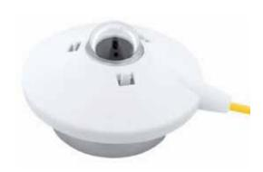
The CMP 3 pyranometer is an instrument for measuring the solar irradiance. The thermopile sensor construction measures the solar energy that is received from the total solar spectrum and the whole Hemisphere (180 degrees field). The output is expressed in W/m2. The CMP 3 pyranometer is designed for continuous indoor and outdoor use.
