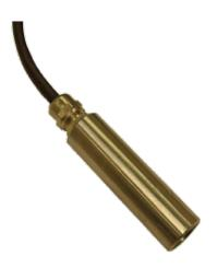
The LMP306 is a highly accurate stainless steel submersible water level sensor that can be connected to iMETOS stations with the precision of +/-0,5% within the measurement ranges. The sensor has an integrated barometric sensor module to increase the precision. Pressure (Measuring) ranges: 0 mWC up to 5 mWC (other distances are available on request). Water level special cable is also available.
